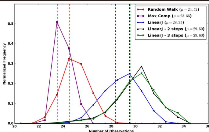
Linear cost function allows the mission to perform more observations due to more convenient slew times on stars with higher completeness values.
