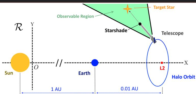
Planar view of the Telescope-Starshade-Target configuration in Sun-Earth rotating frame (not to scale). Starshade aligns with target line of sight (LOS) and suppresses starlight.
