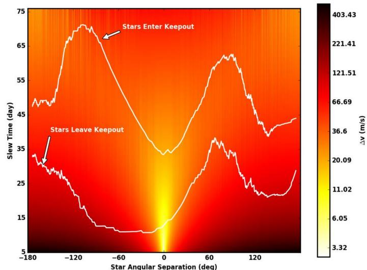
Fuel cost for retargeting maneuvers (slews) between two target stars shown as a function of angular separation of the stars and amount of time needed to transfer. A 2D interpolant is created from this cost matrix to quickly estimate slew fuel costs for any pairs of stars quickly within each decision step of a mission simulation<sup>5</sup>.
