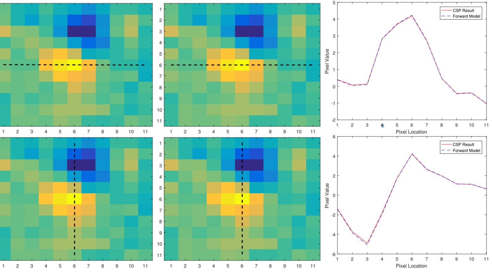
The forward model results compared to the CSP results in one example mode. Top row: horizontal cut. Bottom row: vertical cut. Left column: CSP result. Middle column: forward model result. Right column: pixel comparison.
