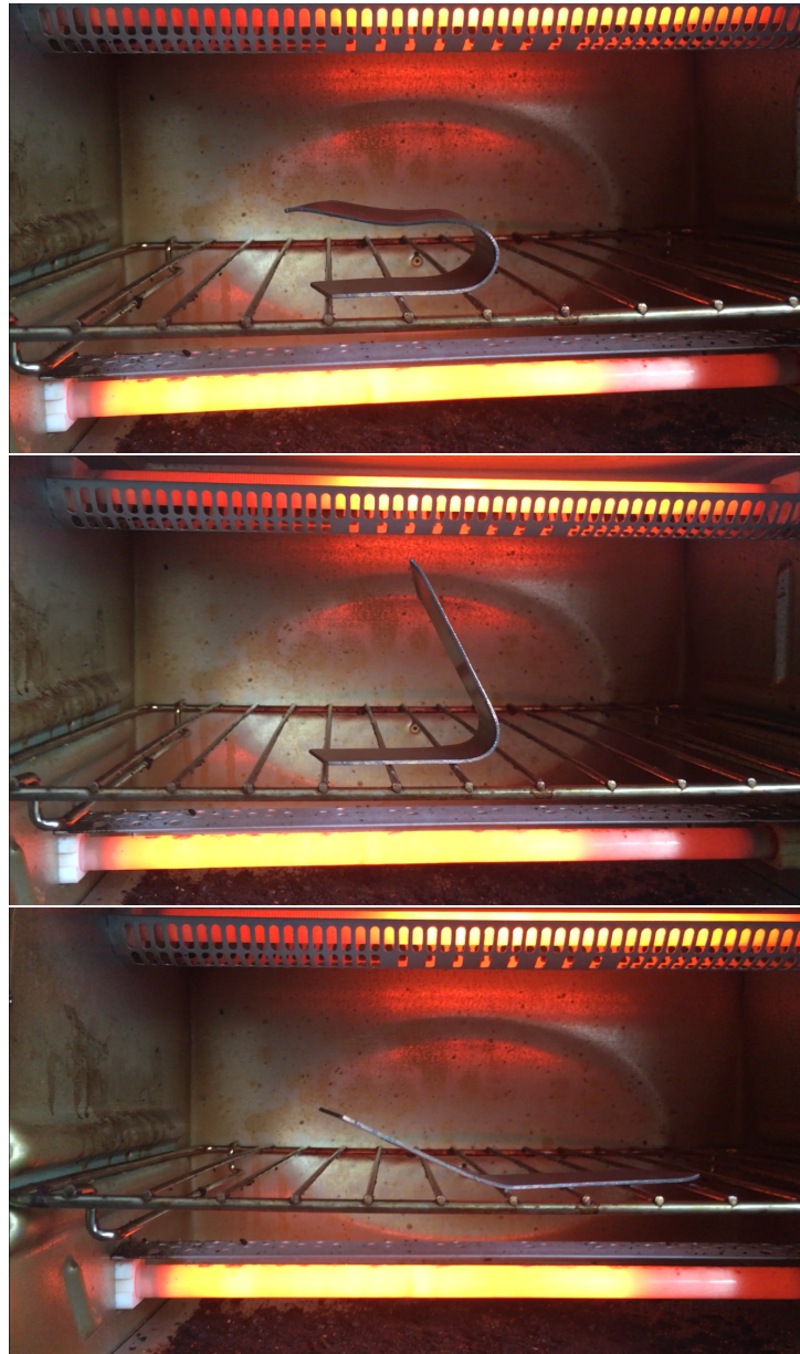
Figure 2: Nitinol specimen transforming into its austenite stage and returning to its original shape. Since this specimen underwent large deformations, it did not return to its complete original shape.
