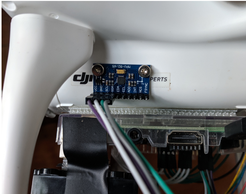
Figure 24: IMU placed on non-level surface on the side of the quadrotor
