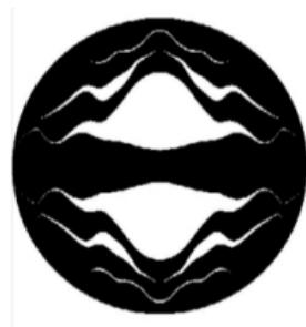
Figure: Pupil mask for high contrast imaging. [Vanderbei et al., 2003]
