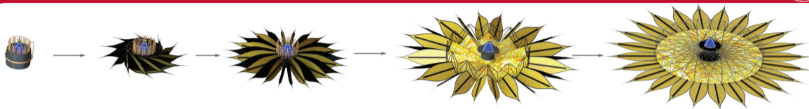
Figure: Starshade deployment concept. Thomson et al. (2011)
